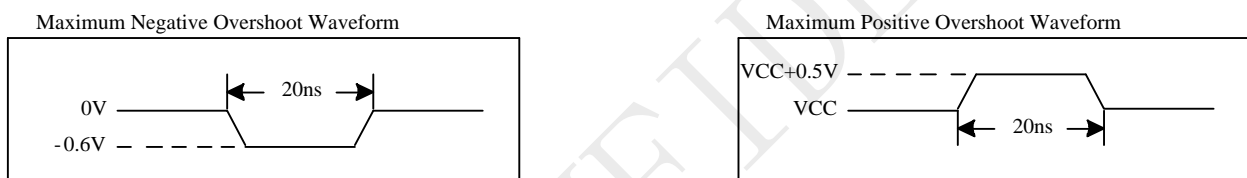
Figure 5-1 Maximum Overshoot Waveform
